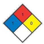
HEALTH 1 Exposure would cause irritation with only minor residual injury (e.g. acetone, sodium bromate, potassium chloride)
