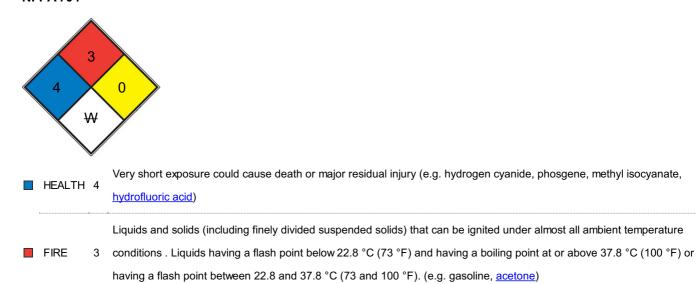
REACT 0 Normally stable, even under fire exposure conditions, and is not reactive with water (e.g. helium, N2)
